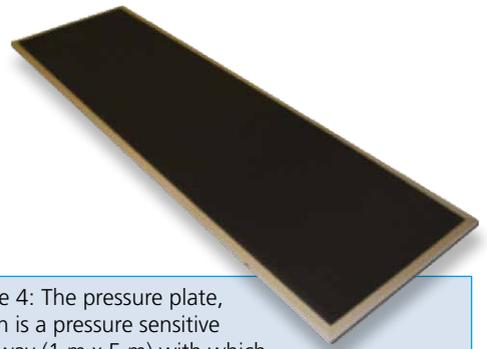
Figure 4: The pressure plate, which is a pressure sensitive walkway (1 m x 5 m) with which gait patterns can be objectively analysed (9,10).
